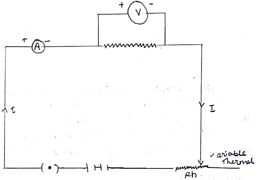
1. Make all the connections properly 'see that positive terminal of battery is connected to the terminal marked + of ammeter and volt meter' Do not leave any connection loose, this adds some indefinite resistance in the circuit. Check the circuit before passing the current in it.
